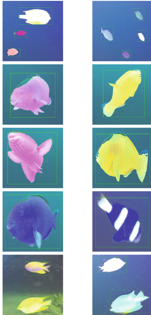
Fig. 3. Sample fish detections with simultaneous bounding box and pixel instance segmentation. The figures above depict sample detections produced by the model. The model simultaneously estimates both the fish object's bounding box (green box outline) and segments the pixels belonging to the fish object within the bounding box. The results above include Dense CRF post-processing which facilitate more accurate segmentation. Segmentation is robust whether the fish object is located in the water column or along the seabed with coral background (i.e. the bottom left picture) (Color figure online)
