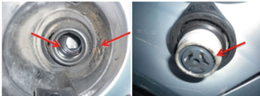
Fig. 7 Black fungal biofilms formed at the inner part of a car fuel tank (left) and internal surface of the lid (right) upon continuous exposure to gasoline vapors. The main strain isolated was identified as the hydrocarbonoclastic species Exophiala xenobiotica . (Courtesy of D. Isola)
