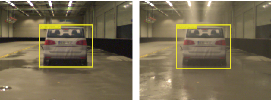
Fig. 6. Object detection without rain (left) and with rain (right). The score decreases from 0.89 to 0.70. The bounding box is shifted to the left by 13 pixels and covers a 6% larger region.
