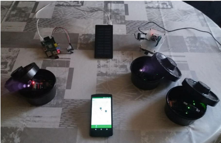
Fig. 6. Complete smart parking prototype test setup.
