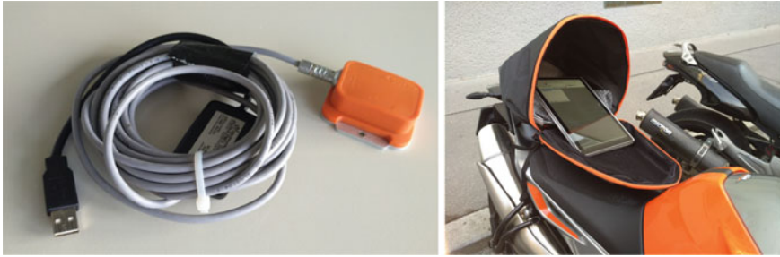
Fig. 1 XSENS sensor and mounting on the motorcycle
