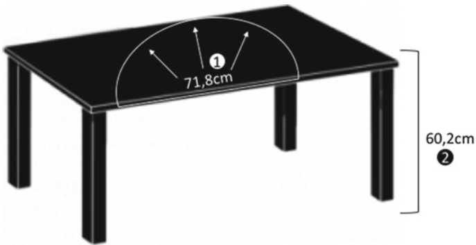
Fig. 2 Dimensions of the workbench according to the Portuguese ergonomic design of seats in order anthropometric data: 1—within reach (maximum); 2—height
