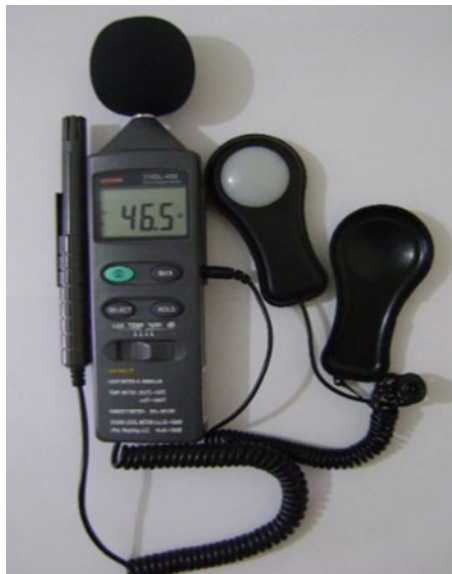
Fig. 2 Thermo-hygro-decibelimeter-luxmeter, model THDL-400
