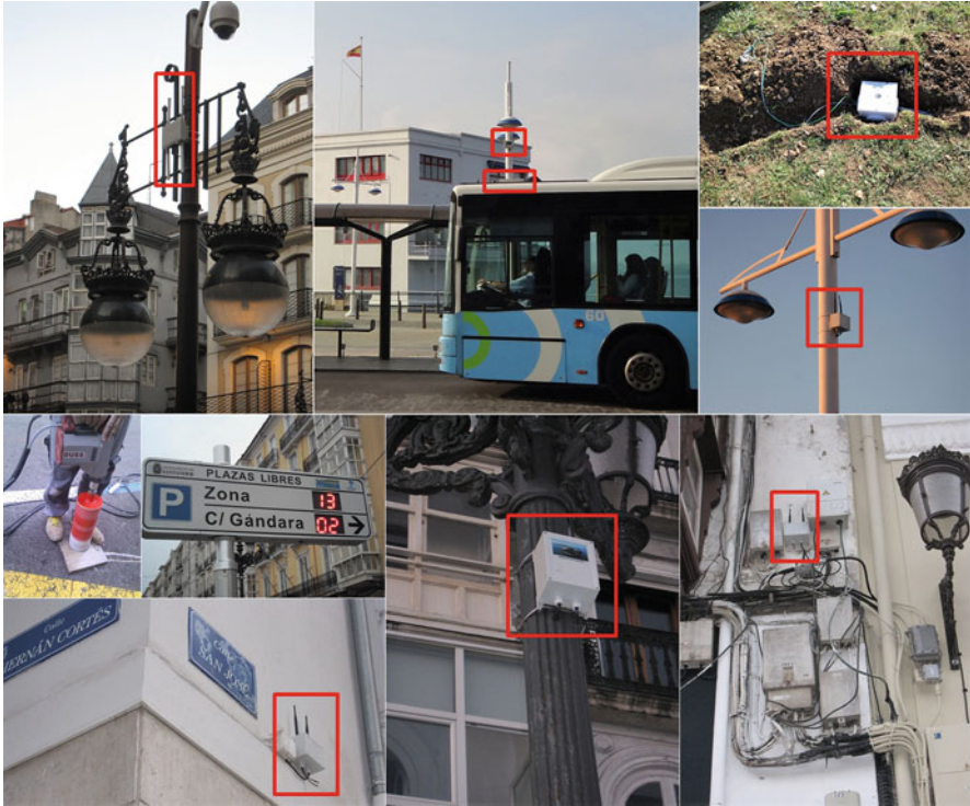
Fig. 2.9 Some examples of IoT devices deployed inside the center of Santander. Both stationary and mobile IoT nodes are used, installed on lamp posts, on top of buses, buried beneath the soil in public parks, or on the walls of buildings at the streets of Santander’s center
