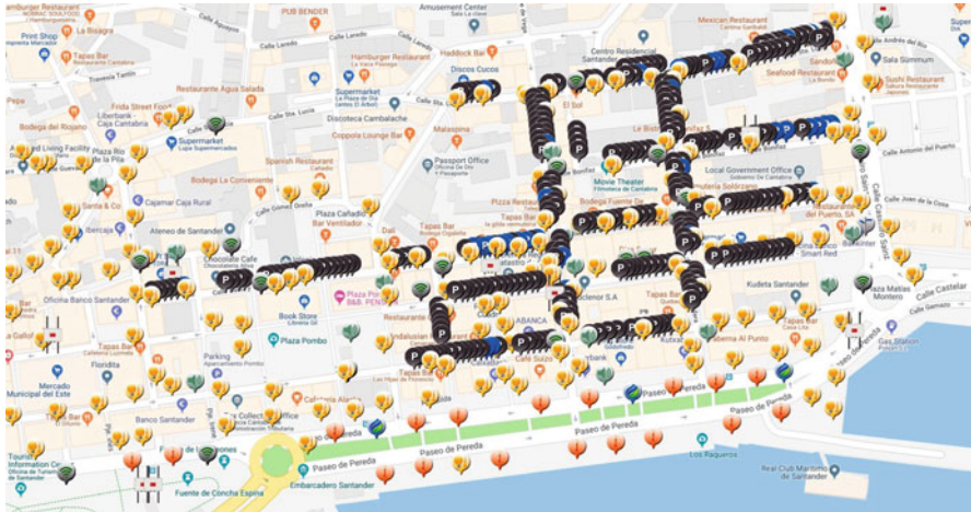
Fig. 2.8 The downtown area in Santander where the majority of the IoT nodes which generate our data sets are installed. It is roughly a 800 by 400 m area in the center of the city, containing parking, noise, weather, traffic, and e-field sensors
