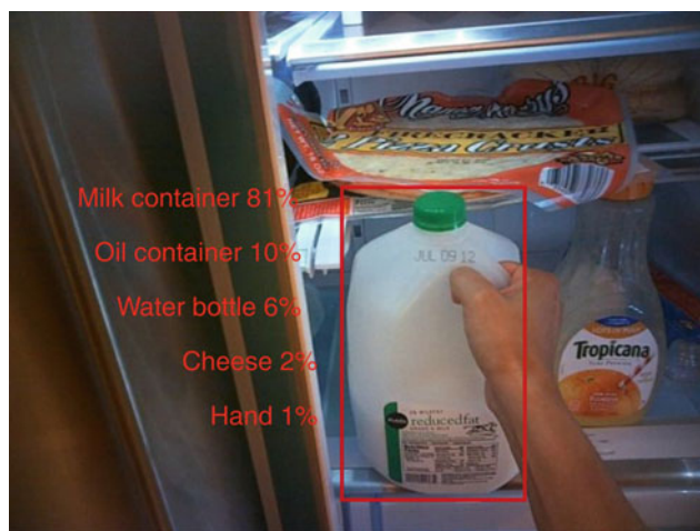
Fig. 3 Sample image from the GTEA Gaze+ dataset with a bounding box inscribing a milk container object. An example of a probability distribution (in percentages) for that bounding box is provided
