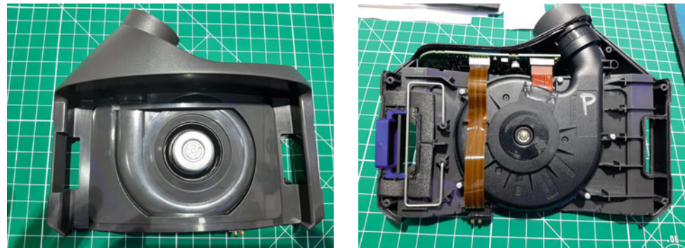
(a) A front view of the blower unit
