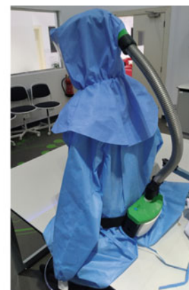
(b) Upgrade air-purifying respirator with UV air sanitizing (COVID-19 compatible)
