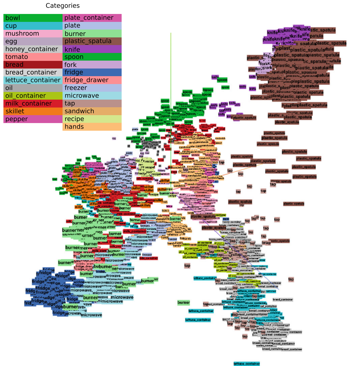
Fig. 9 Feature vectors extracted from the Faster R-CNN represented after a Principal Component Analysis, leaving 3 components. Each class is assigned a colour for a better visualisation
