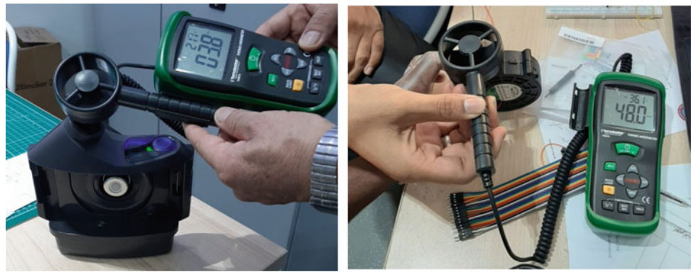
(a) Provide a constant air flow rate of 205 LPM (7.3 CFM) (b) Provide a constant air flow rate of 237 LPM
