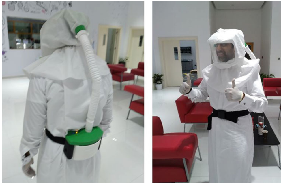
Fig. 20 One of our team wear and test the air-purifying respirator with hood
