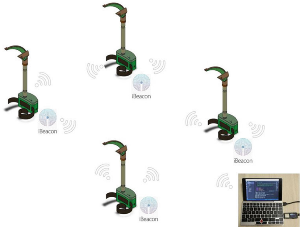
Fig. 15 The architecture of the Bluetooth healthcare staff tracking system
