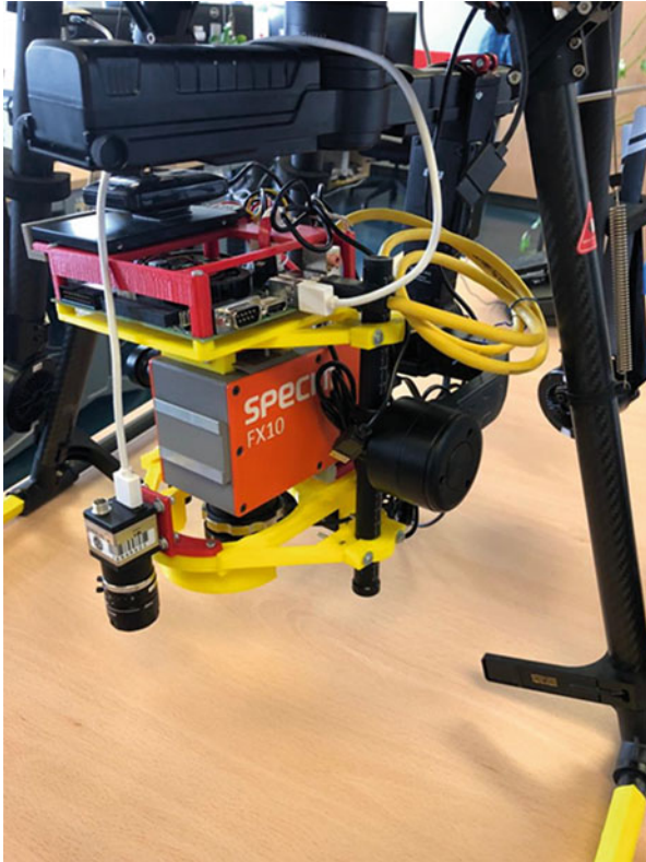
Fig. 5 Detail of the payload of the hyperspectral flying platform
