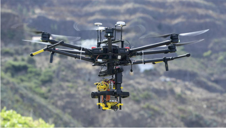
Fig. 4 Hyperspectral flying platform
