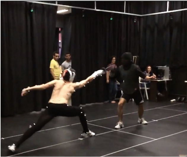
Fig. 2. Lunge motion captured using Optitrack system [9].
