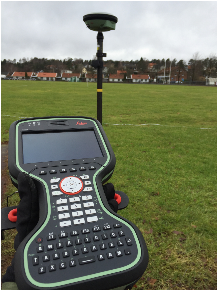
Fig. 4. Surveying of positions using Leica GS14 GNSS antenna and a handheld Leica CS20 controller.
