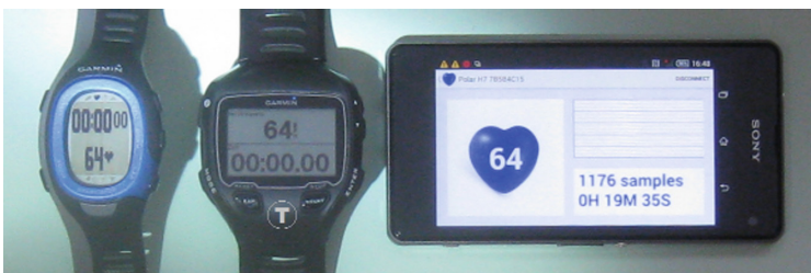
Fig. 2. Sample control units for sports and health supervision: two chest straps with different HR sensors (one ANT+ and one Bluetooth LE), which were attached simultaneously to the same person, feed two sports computers and a smartphone APP with information in parallel. The middle unit marked with T is used in the further investigations here as reference device.
