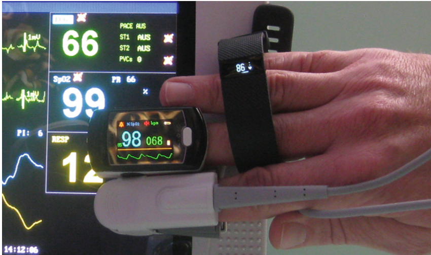
Fig. 9. In this experiment, bracelet unit F was worn intentionally incorrect: despite detached from body skin, it displays blindly a heart rate of 86 BPM, while the three simultaneous medical measures mutually validate a true count that is considerably lower.
