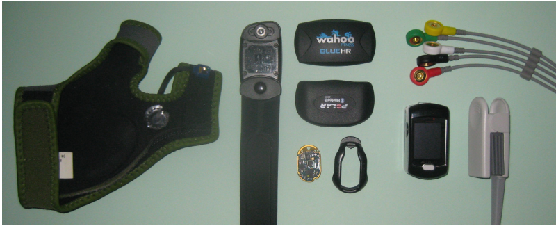
Fig. 1. Examples of sensors for monitoring in health and sports: On the right, an ECG cable set and a pulse oximeter clip for a clinical patient monitor and one standalone finger pulse oximeter are visible; in the middle, three heart rate sensors, one with chest contact strap, and the PCB of 3D footpod sensor with shoe clip are shown; on the left, an early glove product for overcoming the chest strap sensing is displayed that is based on optical measurement at the forefinger.
