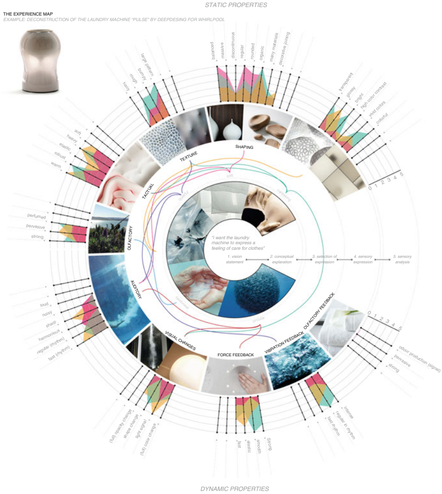
Fig. 4 Example of an Experience Map filled out for the Pulse laundry machine developed for Whirlpool (Camere et al. 2018)
