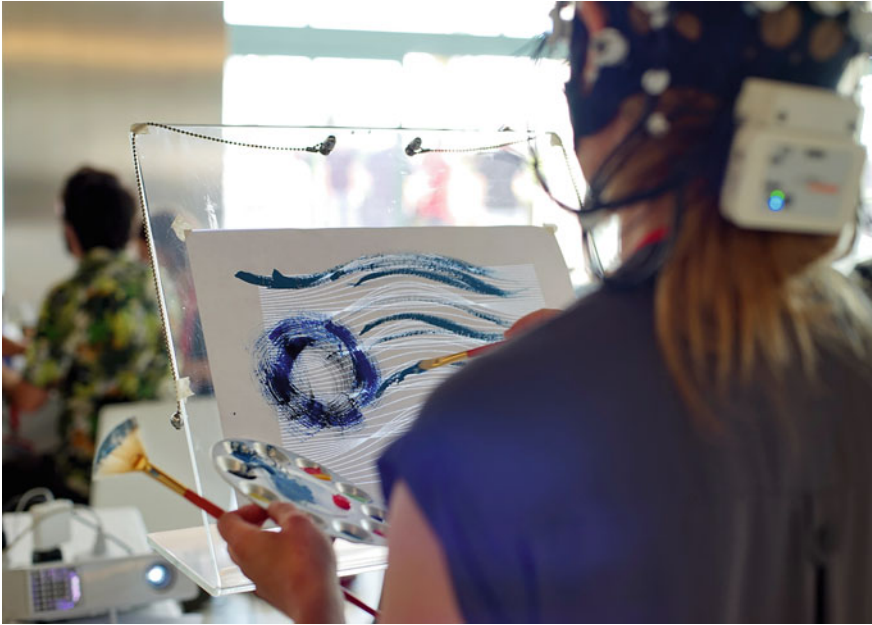
Fig. 12.2 Participant is shown wearing an EEG cap while painting. The purpose of this intervention was to enable creative experience for the BCI system user and to demonstrate how visualization of EEG data could help to enable artistic self-expression. Active EEG analysis was combined with visual neurofeedback output to enable a process that replicated methods of traditional analog painting. The finished product consisted of visual overlays projected upon a transparent canvas (Photograph by Lukas Gehrke, Valencia, Spain, 2017)
