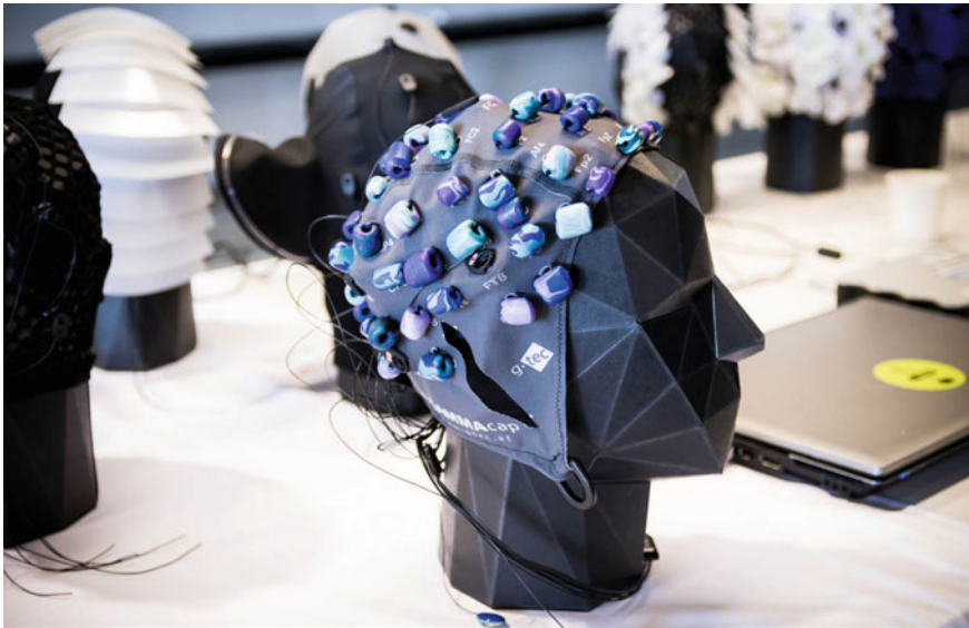
Fig. 17.13 Another kids’ team developed this design based on beads. The beads cover the electrodes and could make the cap more cosmetically appealing to kids, especially kids who like beads
