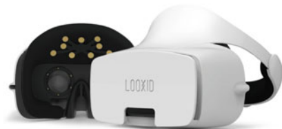
(b) EEG electrodes integrated in the LooxidVR headset.
