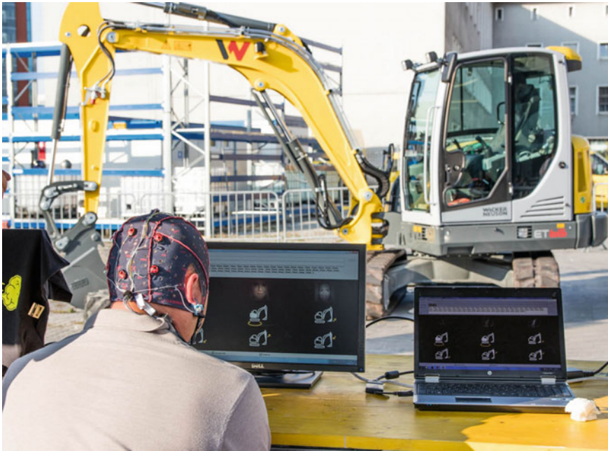
Fig. 17.9 A hacker uses a P300 BCI to control heavy equipment. The different commands on the screen reflect different instructions
