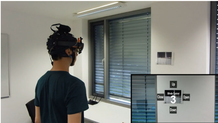
Fig. 16.5 Room control via AR using the SSVEP-BCI paradigm
