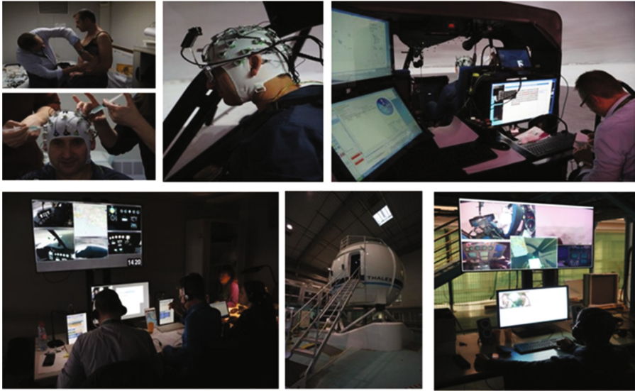
Fig. 2. Above on the left, installation of the sensors. The electroencephalogram was not used for the model. It serves as measure control. Top right, an internal view of the simulator with the simulator operator. Below on the left, the Human Factor expert and the expert pilot. Bottom center, the simulator. Bottom right the data quality control station
