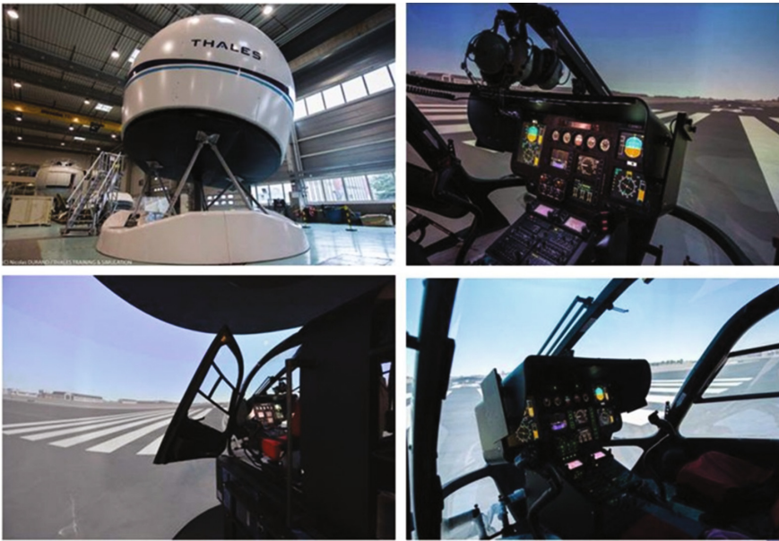
Fig. 1. Full flight simulator with EC 135 helicopter cockpit (Thales ©).
