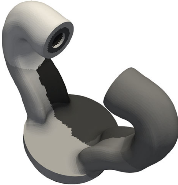
Fig. 14.7 A complicated surface with open geometric edges
