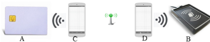
Fig. 1. Schematic diagram of basic relay attack setup
