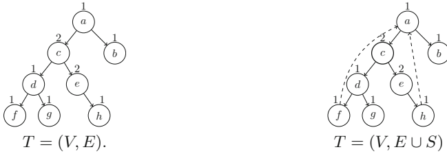
Fig. 2. Example of Algorithm 1. Consider the node c with w_c = 2 , p_v = 1 \forall v \in V and B = 2 . We have: g(d, 2) = 19 , g(d, 1) = 12 , g(e, 1) = 7 + 2(6) = 19 . Therefore g(c, 2) = g(e, 1) + g(d, 1) + w_c \cdot (p(T(r)) - p(T(v))) = 35 .
