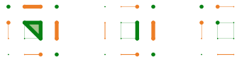
Fig. 6. Total contribution to the Euler-Poincaré characteristic in a grid cell including the shares of intersections with neighbor cells. Left. the cell contribution to the Euler-Poincaré characteristic for itself is 1. The intersection is non-empty in the four edges. The contribution of each one is -1 , shared by two cells. The intersection is non-empty in three vertices. The contribution of each one is 1 , shared by four cells. The global measure for the cell is then \chi = 1 - 4 \times \frac{1}{2} + 3 \times \frac{1}{4} = -\frac{1}{4} . Middle. \chi = 1 - 3 \times \frac{1}{2} + 2 \times \frac{1}{4} = 0 . Right. \chi = 1 - 2 \times \frac{1}{2} + 1 \times \frac{1}{4} = \frac{1}{4} .
