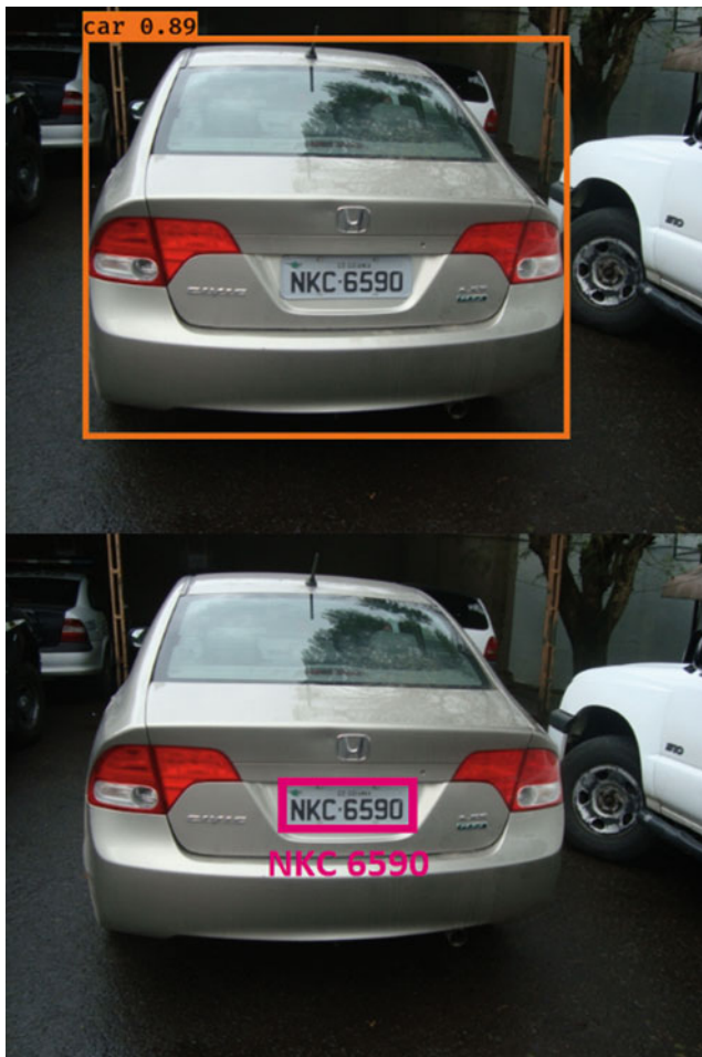
Fig. 65.7 Results collected. (top) The result from SSD. (bottom) The result from OCR
