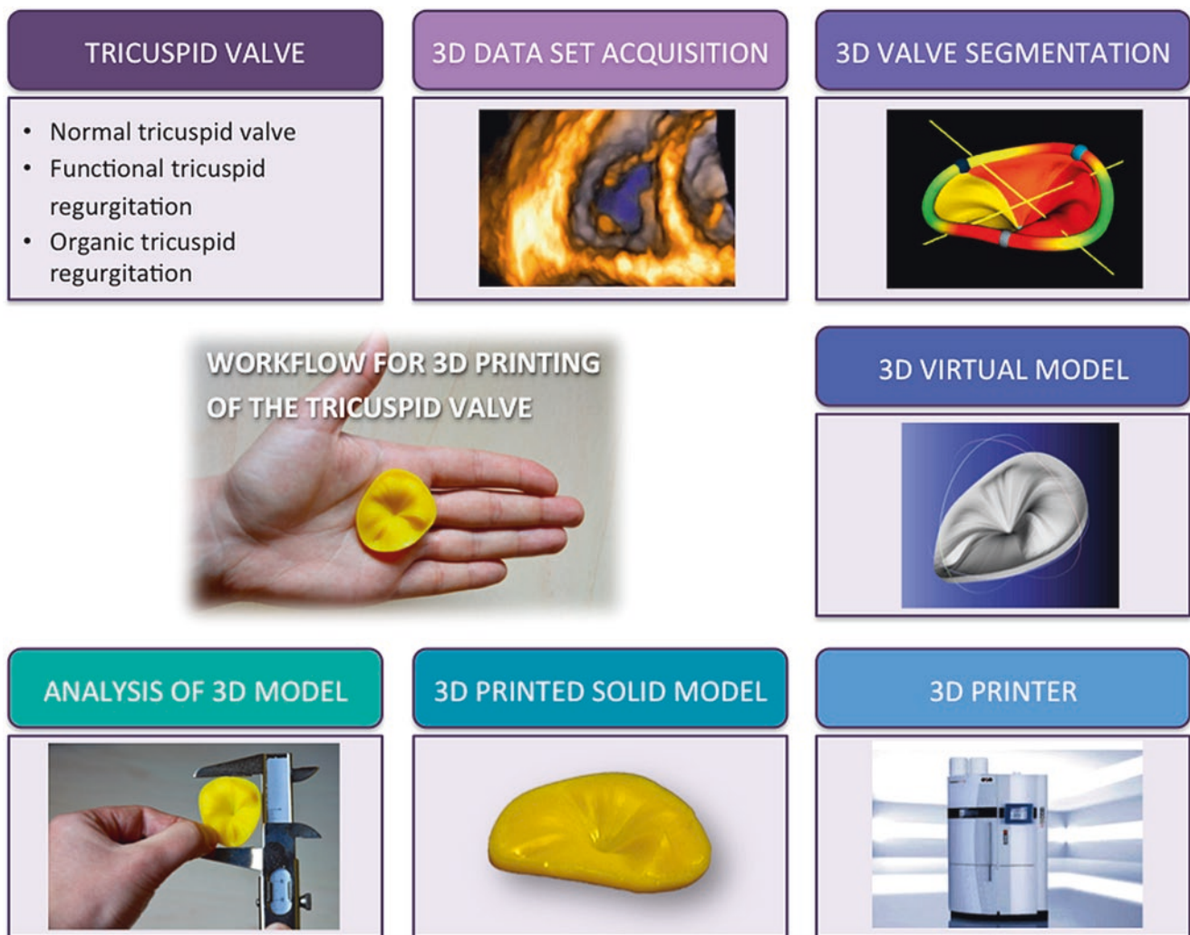
Fig. 2.15 Workflow associated with printing a 3D solid model of the tricuspid valve. A sample of workflow is shown diagrammatically from the transthoracic acquisition of the three-dimensional echocardiography data set, to its segmentation, creation of a virtual 3D model and stereolithographic file that can be printed using any commercially available 3D printer. The 3D solid model of the valve can be used to appreciate valve morphology and perform qualitative and quantitative analysis
