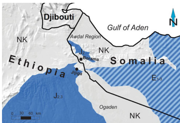
Fig. 1 Distribution of major karstic formations and aquifers of Somalia and Ethiopia (modified from authorised inputs of Stevanovic and Kebede for WOKAM—World Karst Aquifer Map 2017). Legend: NK—non-karstic rocks (Precambrian granites and crystalline rocks, Cretaceous Yessoma Fm. sandstones, Tertiary and Quaternary sediments and basaltic rocks); J 2,3 —Middle and Upper Jurassic carbonate rocks; E 1,3 —Eocene evaporates and carbonates
