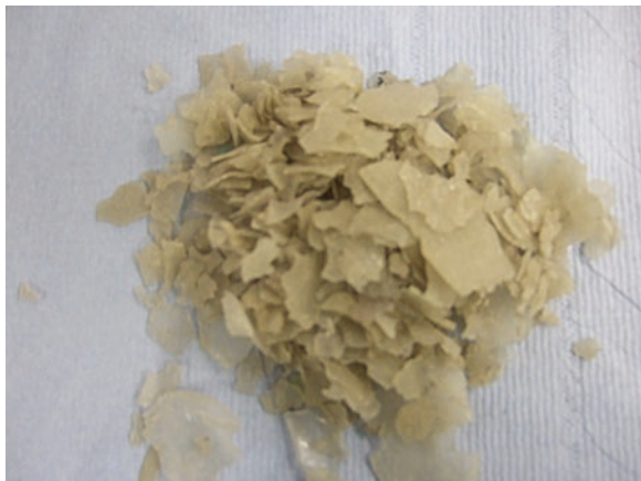
Fig. 4.2 Polyvinyl butyral film as a part of safety windscreen [8]
