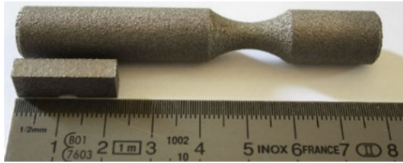
Fig. 14.3 Standard versus miniature as-built fatigue specimens
