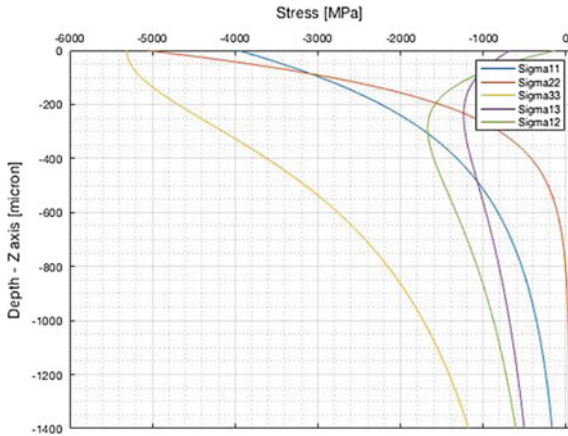
Fig. 41.2 Stress distribution in case of no microinclusions
