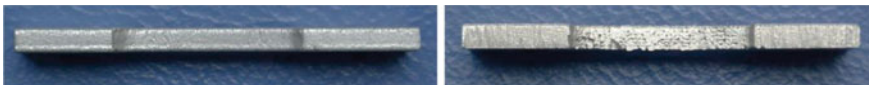
Fig. 15.2 Surfaces of an AlSi10Mg specimen built in the X direction: as-built state (left) and after the removal of support structures (right)
