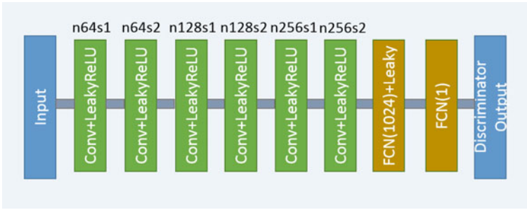
Fig. 14.2 The structure of the discriminator network. n and s have the same meaning as in Fig. 14.1
