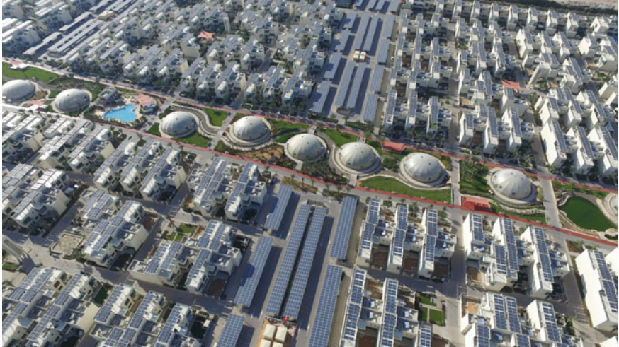
Fig. 4.2 Aerial view of The Sustainable City showing solar rooftops and solar car parks, which help reduce utility bills
