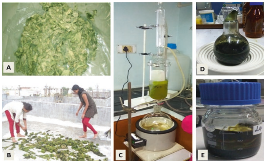
Fig. 5 (a) Harvested algal biomass, (b) sun-drying of algal biomass, (c) Soxhlet extraction of lipid, (d) unpurified lipid, (e) purified lipid
