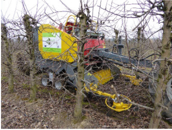
Fig. 7 Big baler for pruned biomass baling strategy [19]
