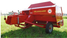
Fig. 8 Baler producing rectangular bales (Source www.lerdaagri.com )
