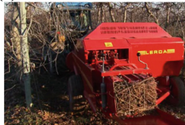
Fig. 8 Baler producing rectangular bales (Source www.lerdaagri.com )
