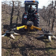
Fig. 5 Options for windrowers attachment to improve pruned biomass harvesting process
