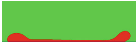
Fig. 11.6 Although the equilibrium contact angle of the substrate is \theta = 150^\circ splashing does not occur for an oblique impact on a smooth substrate with the impact parameters We_n = 140 and \Phi = 30^\circ
