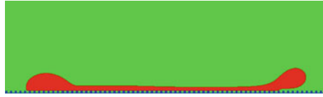
Fig. 11.9 Simulation result for an oblique impacting droplet with an impact angle of 30^\circ and normal Weber number of 140. The equilibrium contact angle of the substrate is \theta = 110^\circ . The numerical results show that the splashing vanishes with an increase in wettability of the substrate to \theta = 110^\circ
