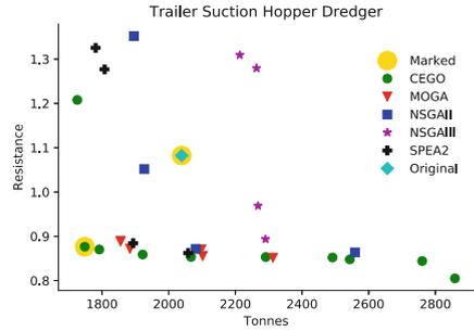
**Fig. 5.** Original design and Pareto front obtained by the five algorithms on dredger case.
