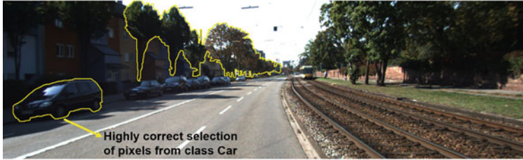
Free-form or polygon selection of objects for labeling in a video frame.
