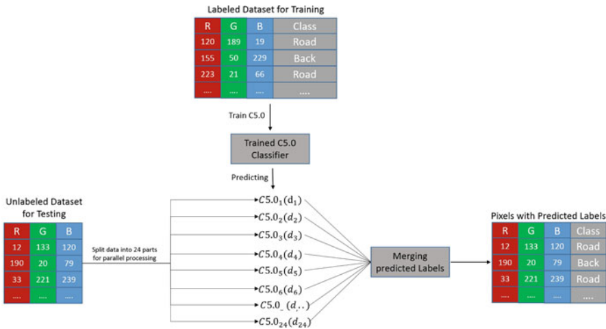
Fig. 6.8 Block diagram of C5.0 decision tree classifier execution in parallel
