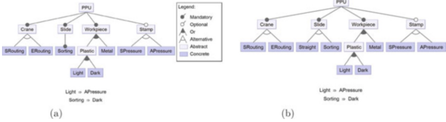
Fig. 7.12 Feature-model evolution scenarios. (a) Feature model version 2. (b) Feature model version 3
