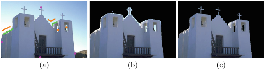
Fig. 1. (a) Original image with four extreme points (magenta) for the method in [12] and orange and green markers for the proposed algorithm. (b) Result of the method in [12] with errors and (c) the desired segmentation using the proposed algorithm. (Color figure online)
