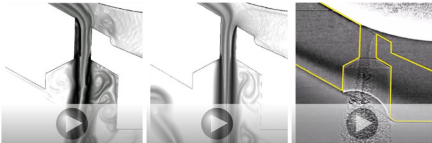
Fig. 12 Results of a shorter injector. Left ( https://youtu.be/KHDVURSKY3M ): Density gradients of a simulation using existing cavitation/hydraulic flip models. Center ( https://youtu.be/MQKjlsv57ow ): Density gradients of a simulation using improved cavitation/hydraulic flip models. Right ( https://youtu.be/wkivdPoBn3c ): X-ray measurements [8]
