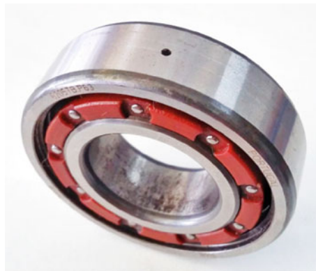
Fig. 8.5 Bearing element with artificial damage in the outer race
