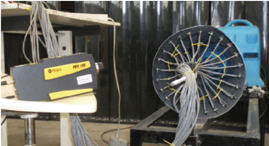
Fig. 2.4 Rotor: setup and laser vibrometer used for calibration
