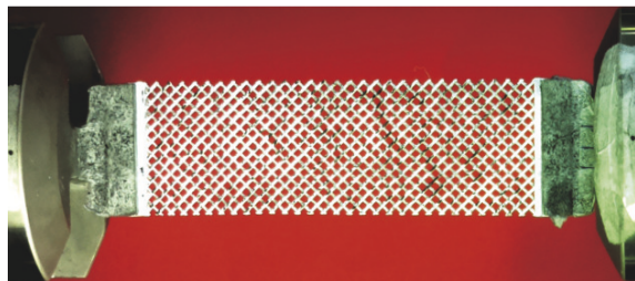
Fig. 33.3 Shot of a pantographic lattice with orthogonal fibers inside a testing machine immediately before an elongation test.
