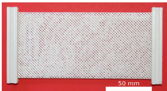
Fig. 15.1 In-house manufactured specimen made out of polylactic acid (PLA): Metamaterial with pantographic substructure (Sample A ).
