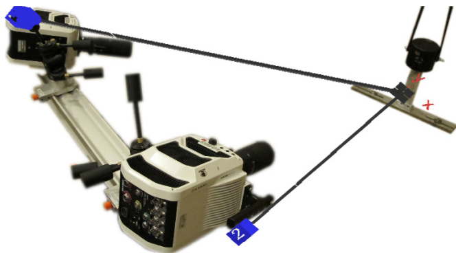
Fig. 19.2 3D reconstruction of the camera setup operated by the DIC software, overlaid to a picture of the real setup.
