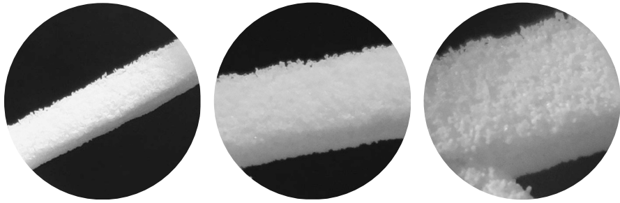
Fig. 33.6 Blow-up sequence of a pantographic lattice part built by a 3D printing process using polyamide powder; the sequence clearly shows the granular nature of the specimen.
