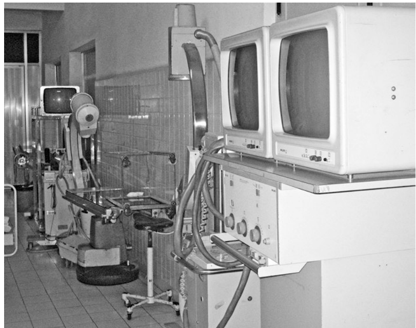
Fig. 7.6 Two unusable, donated C-arms clutter the limited hall space in a Cambodian hospital. They cannot be fixed or disposed of locally due to the radioactive components
