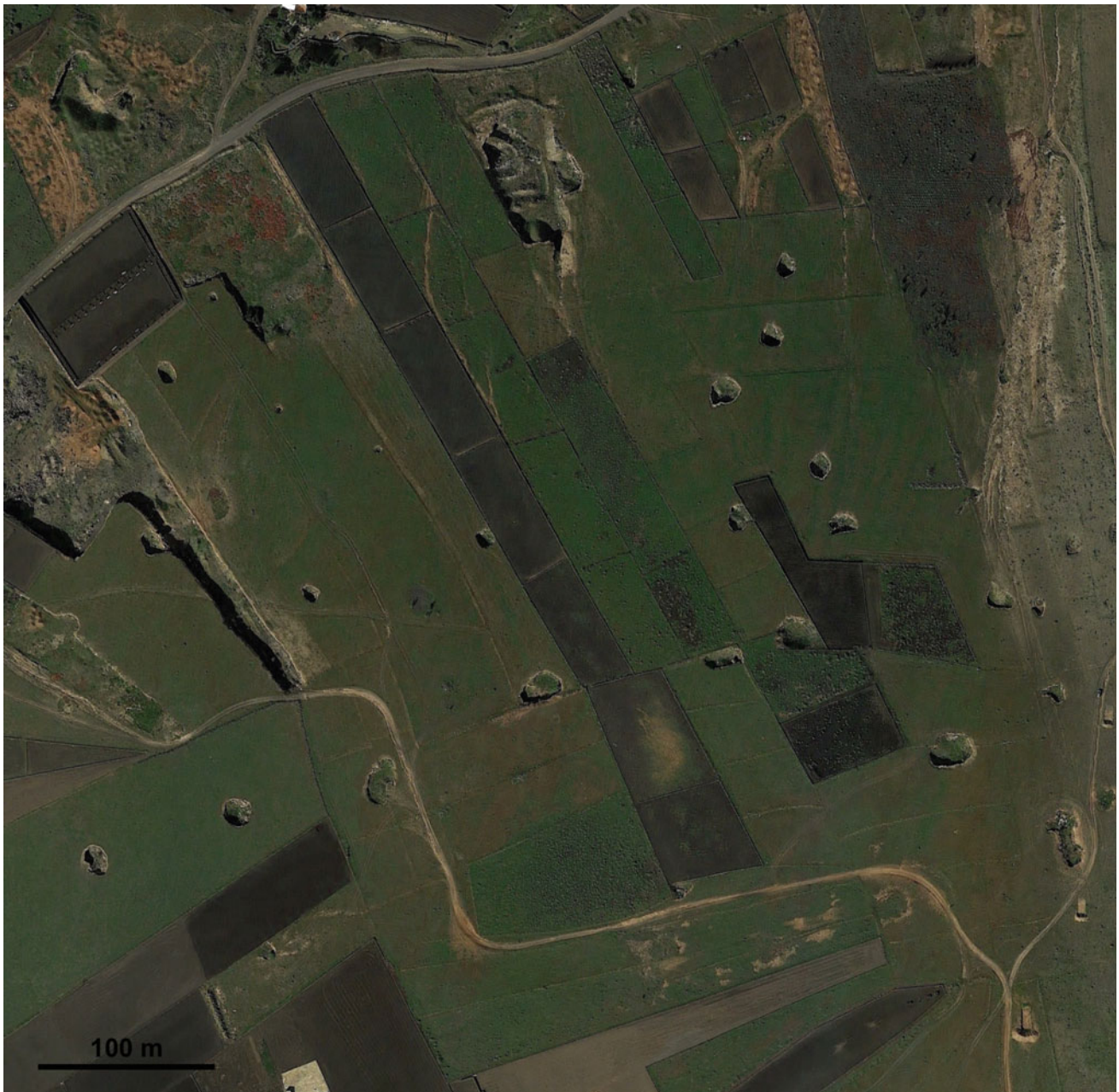
Fig. 4 Sinkholes in pyroclastic terrains in Lomo de San Andres near Mozaga, probably related to piping processes in unconsolidated pyroclasts below a harder substrate. The process could have been
