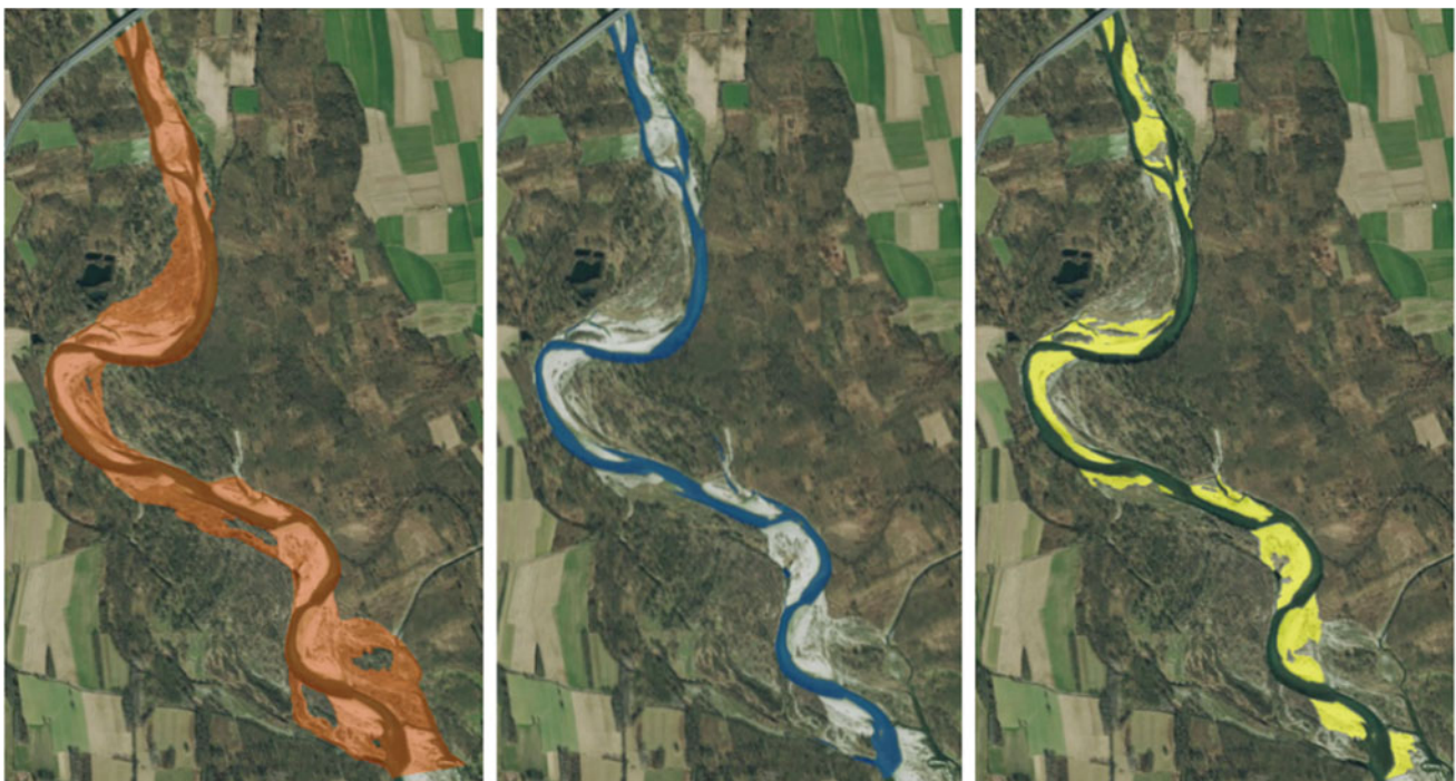
Fig. 2 River features extracted from SAR and overlaid to orthophoto. From left to right: Active Channel (AC), Water Channel (WC), Sediment Bars (SB)
