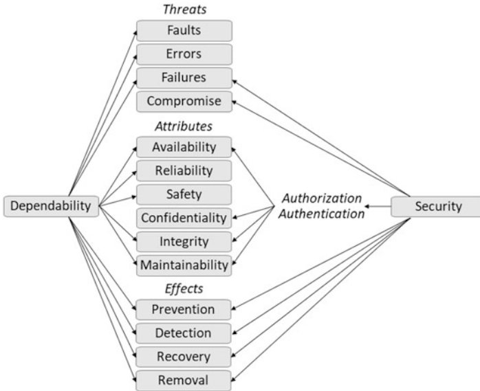
Fig. 6.2 Related concerns for dependability and security in CPS (adapted from [4])
