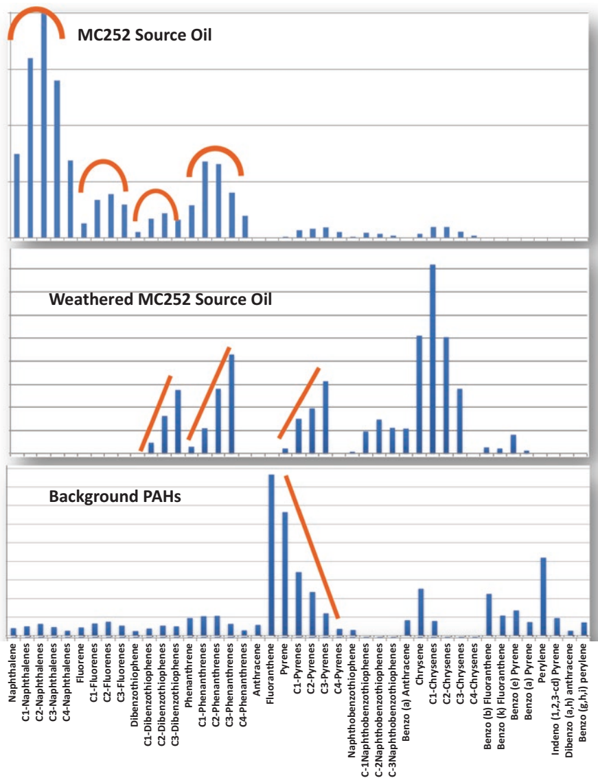
Fig. 3.6 Distribution of PAH compounds in MC252 source oil, weathered MC252 oil residues, and a coastal sediments with no oil residue contamination (no hopane biomarkers) – differentiation between petrogenic and pyrogenic sources of PAHs by alkyl homologs abundance. The red lines represent a typical distribution of parent and their alkylated homologs in petroleum vs pyrogenic sources
