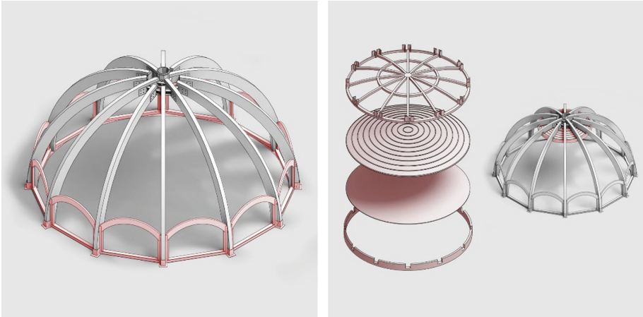
Fig. 5. Frame's perimeter completion and central spherical cap addition
