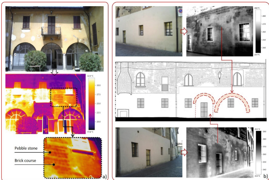
Fig. 3. Examples of thermographic analysis for the masonry texture detection and the integration with the historical sources for interpreting the evolution of the buildings
