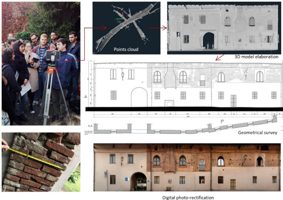
Fig. 1. Example of geometric survey activity based on laser scanner and common measurements, implemented with image rectification.
