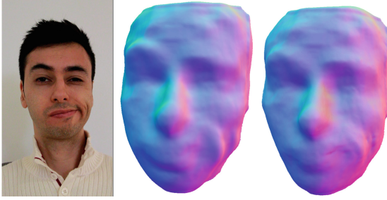
Fig. 5. Comparison of NRST’s reconstruction (right) and the one of Yu et al. [43] (middle). It becomes obvious that both capture the facial expression shown in the input frame (left), but the proposed approach is significantly faster than the one of Yu et al. due to our data-parallel GPU implementation.
