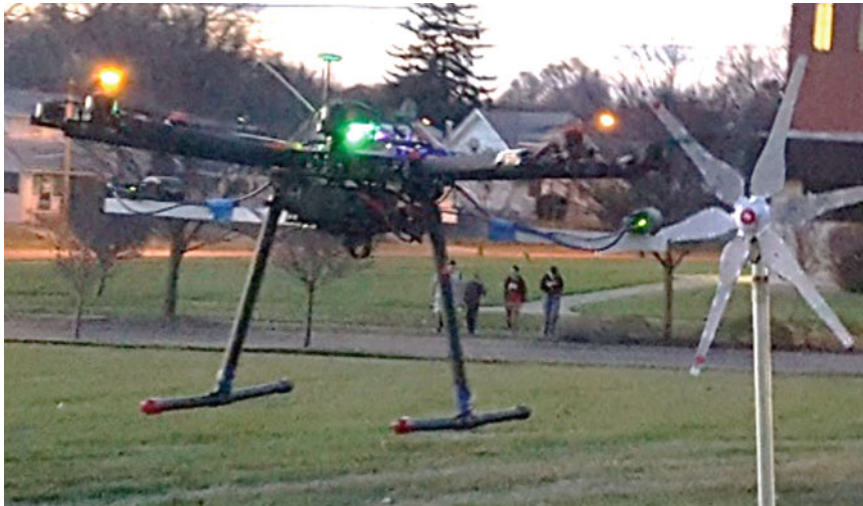
Fig. 9.8 Flying drone for capturing images of the wind turbine blades
