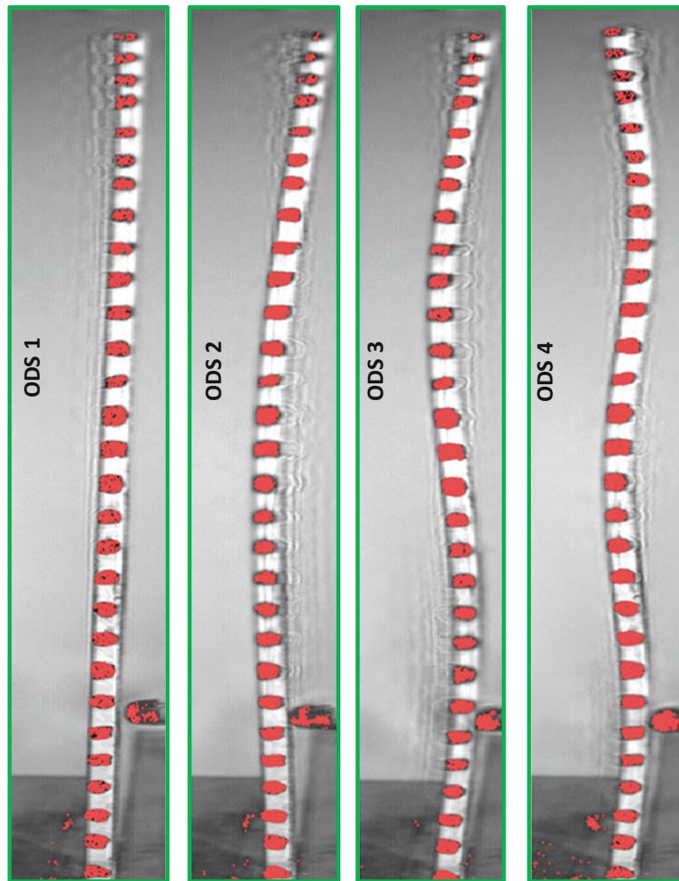
Fig. 8.3 Tracking the targets in motion-magnified videos using the particle filter algorithm
