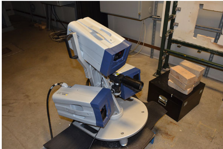
Fig. 12.1 Polytec PSV500 Assembly and high definition video camera
