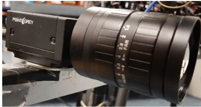
Fig. 9.3 Point Grey GS3-U3-32S4M-C camera with Fujinon 1:1.4/12.5 mm CF12.5HA-1 lens
