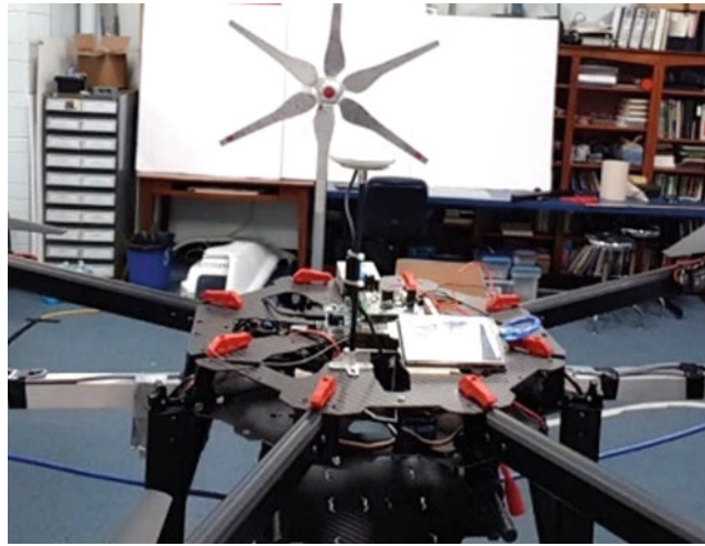
Fig. 9.5 Indoor laboratory test setup to measure vibrations of wind turbine
