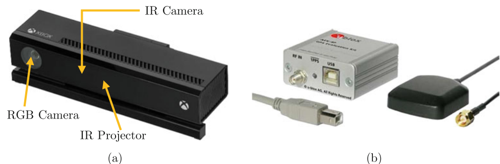
Fig. 1 The devices used in this work: (a) Kinect v2 device with underlined the three imaging sensors, (b) low-cost u-blox GNSS receiver
