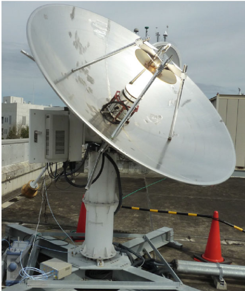
Fig. 2 MARBLE with 2.4 m dish and the NINJA feed
