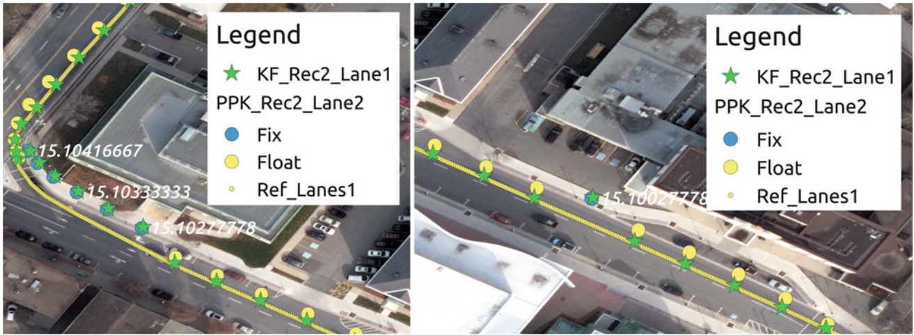
Fig. 6 Wrong filter positioning due to a wrong GNSS position fixes on a urban canyon
