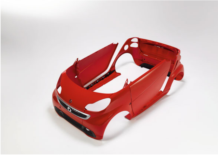
Fig. 6.44 Body of the Smart ForTwo produced from colored PP Daplen EF150HP (Borealis AG)
