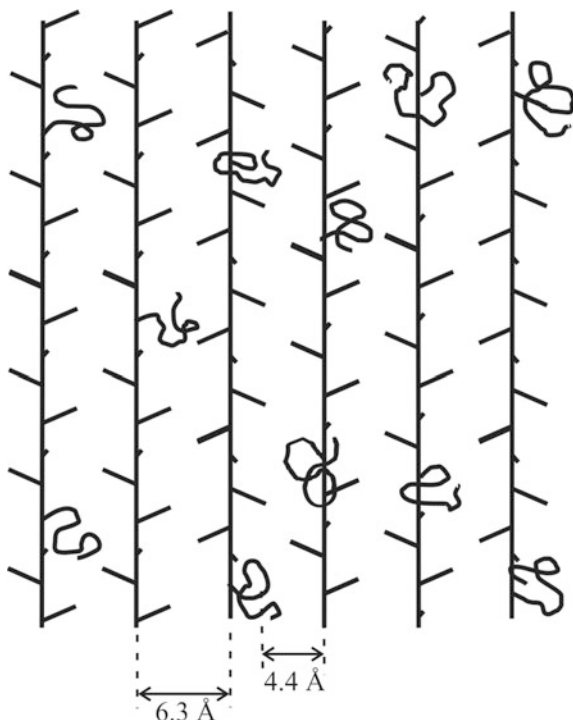
Fig. 2.25 Schematic model of the organization of chains of iPPOct copolymers in the mesophase. Reprinted with permission from Ref. [56]. Copyright 2010 by the American Chemical Society
