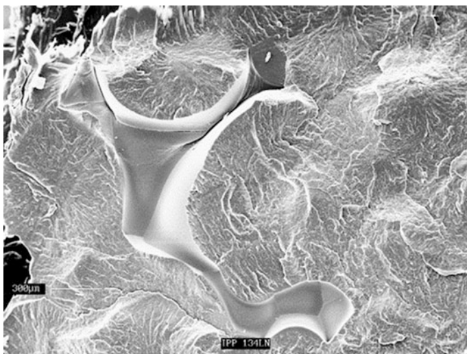
Fig. 4.25 Scanning electron micrograph of fracture surface of iPP thick plate crystallized isothermally at 134 °C; large cavities between spherulites are visible. Authors own micrograph
