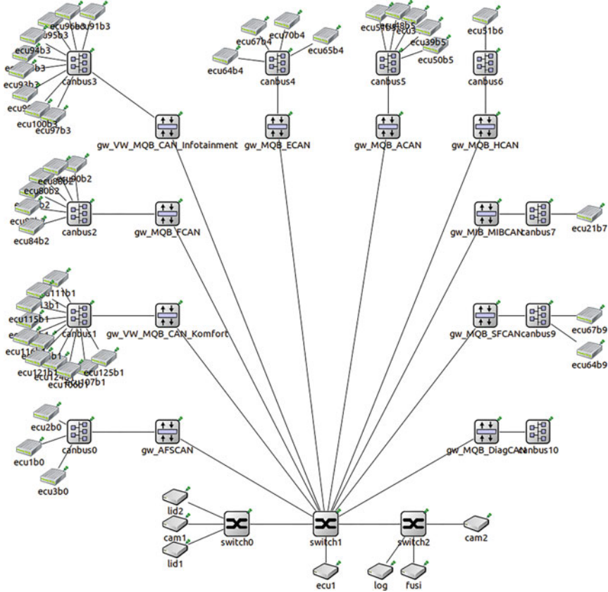
Fig. 10.12 Ethernet backbone within the RECBAR car
