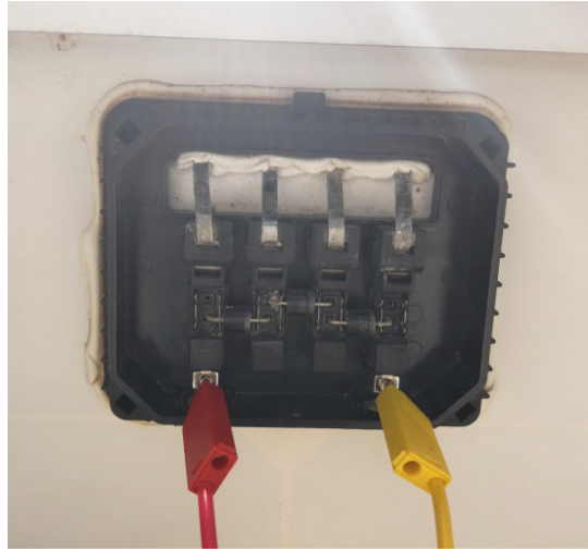
Fig. 9. Module junction box open, showing the conducting strips which connect the bus ribbon to the bypass diode terminal, three bypass diodes and the terminals for the connection for the PV terminals.
