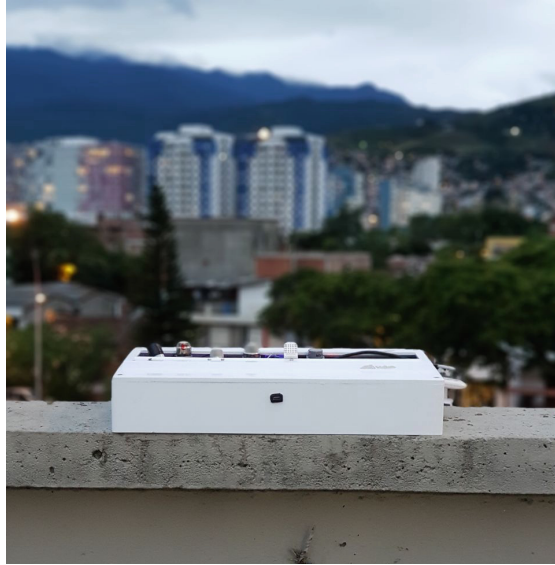
Fig. 6. Image of one of the air quality monitoring prototypes.
