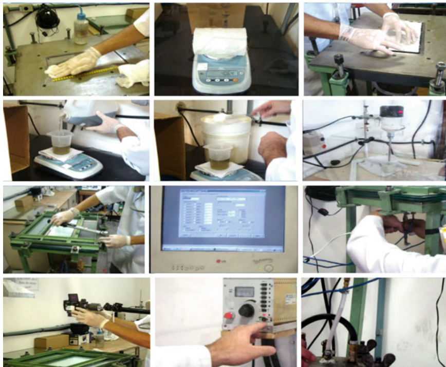
Fig. 3.2 Basic steps for RTM experiment
