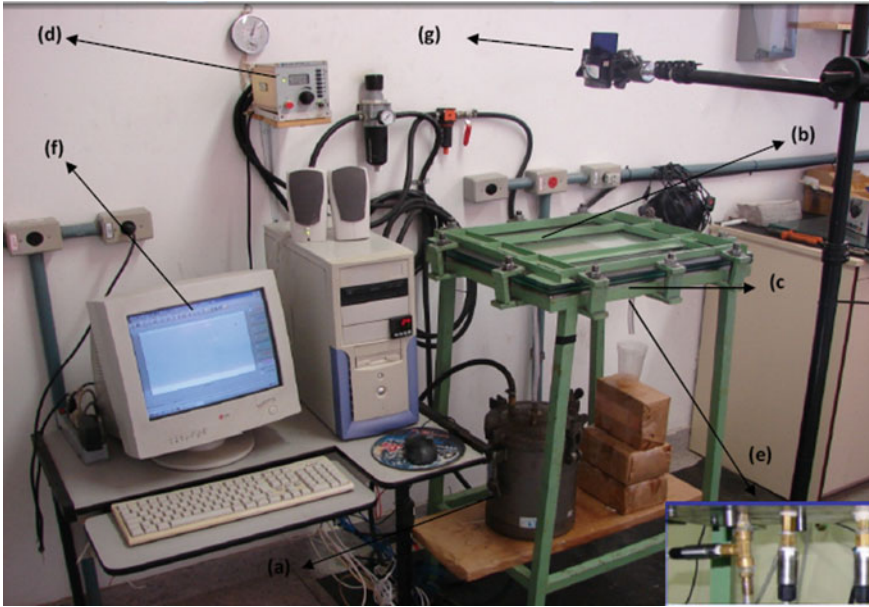
Fig. 3.1 Photo of the RTM experimental apparatus available at LACOMP/Federal University of Rio Grande do Sul (Brazil): a pressure vessel, b strengthened glass top mold, c steel lower mold, d pressure controller, e pressure transducers, f data acquisition system and g camera
